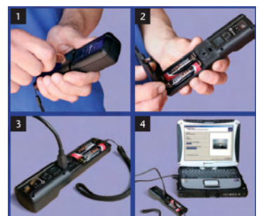
Downloading files is easy - open the rear of the camera using a coin to access the USB port. Then simply connect the camera to any PC and downloading begins automatically.
